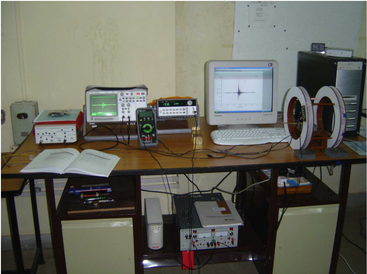
Figure 2.11: Photograph of the experimental set-up for measuring Magnetic Barkhausen noise.
