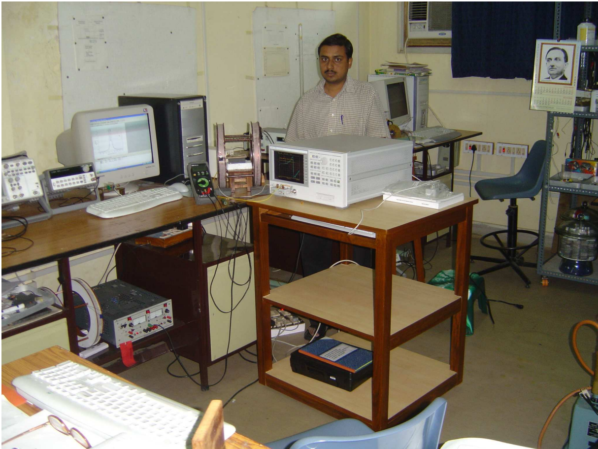
Figure 2.9: Photograph of the experimental set-up for measuring giant magnetoimpedance.
