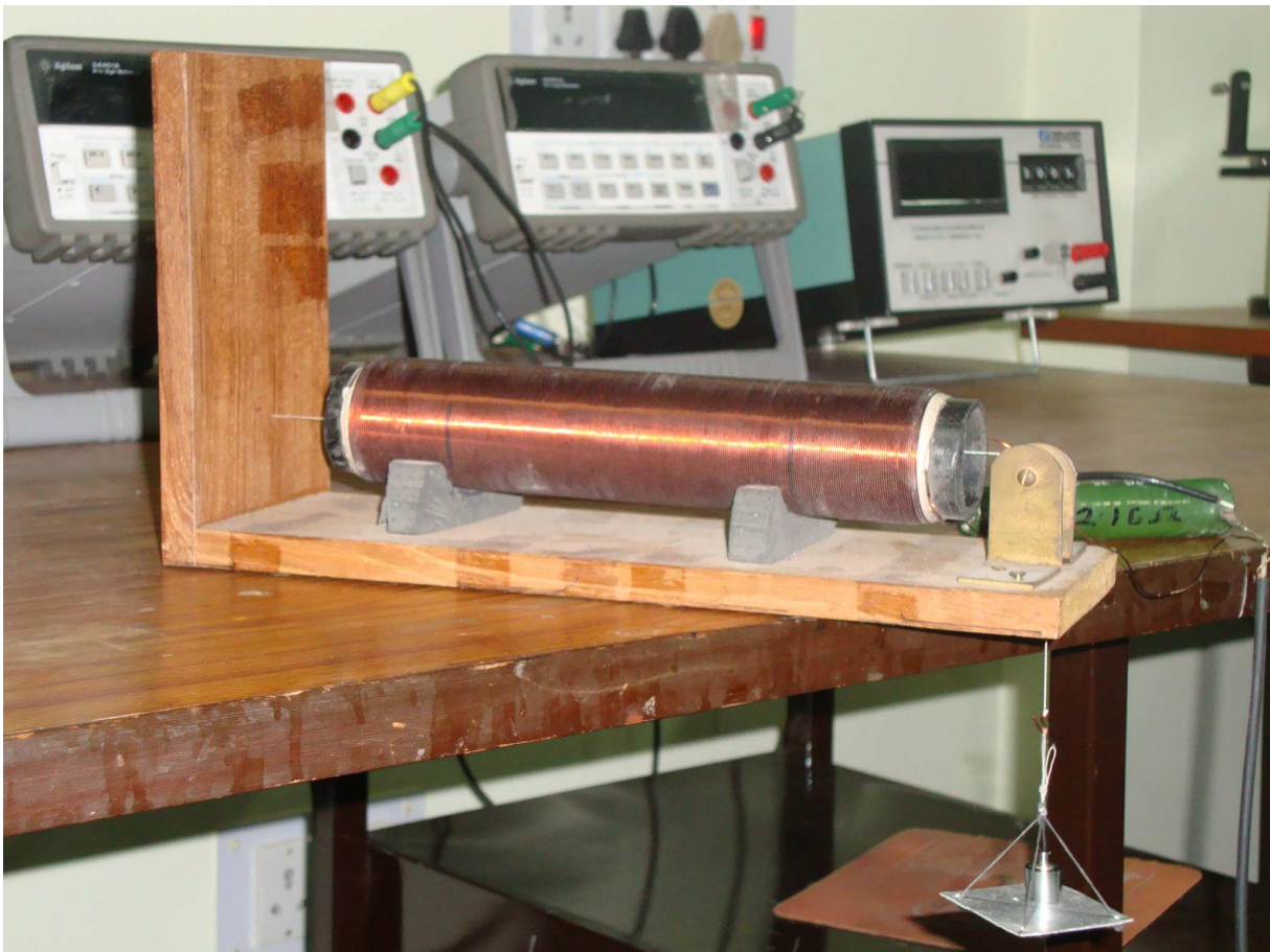
Figure 2.7: Photograph of the experimental set-up for studying stress dependent magnetization measurements.
