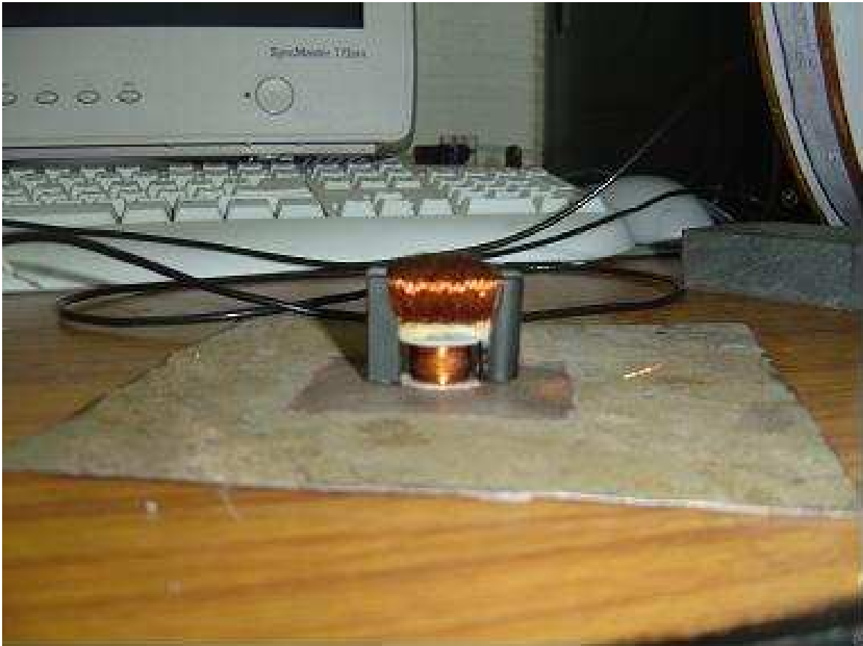
Figure 2.13: Photograph of a U-shaped ferrite core with the pick-up coil placed between the pole pieces of the U-core magnet used for measuring surface Magnetic Barkhausen noise.
