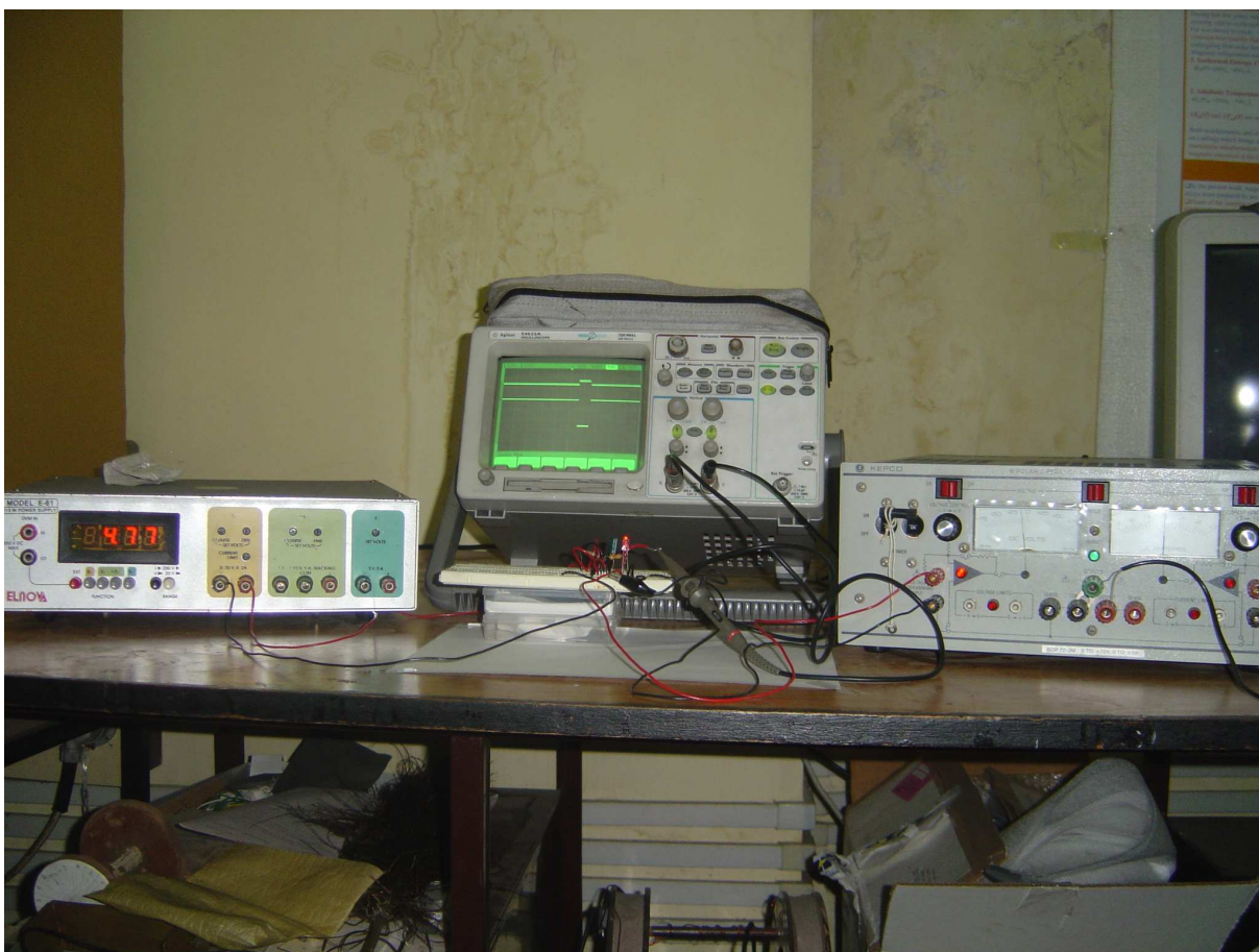
Figure 2.15: Photograph of the experimental set-up for flash annealing.
